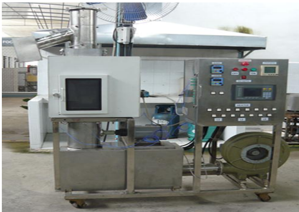
Production of Instant Rice using Combined Microwave Vibro-Fluidized Bed Drying
