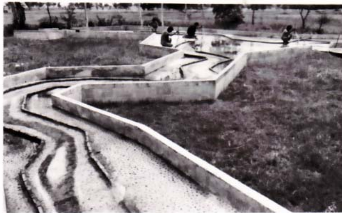
Flood Pattern and Potential Scour Downstream of Mae Ngat Dam Spillway, Mae Ngat Dam Project - Thailand
