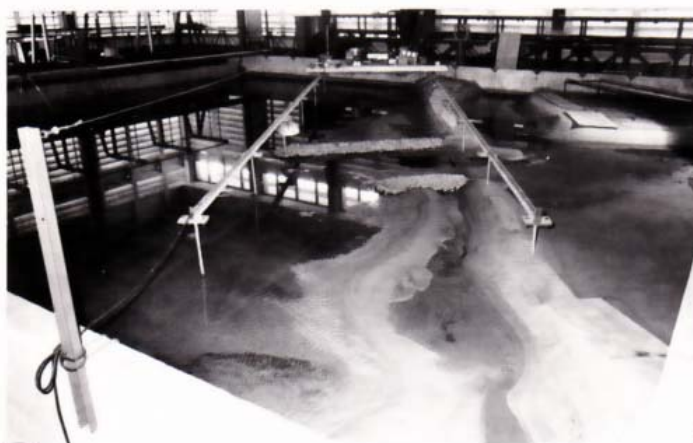
Hydraulic Model Study of Rayong River Mouth
