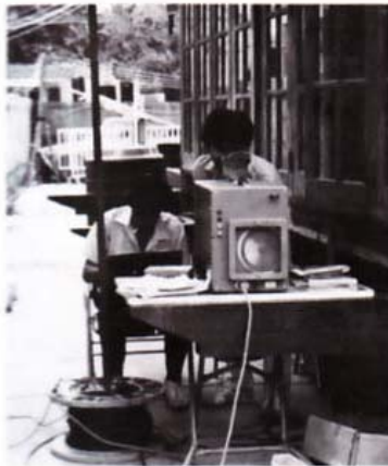
Measurement of pile vibration by Geotechnical and Transportation Engineering students.
