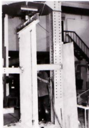
Testing an Insucrete panel
