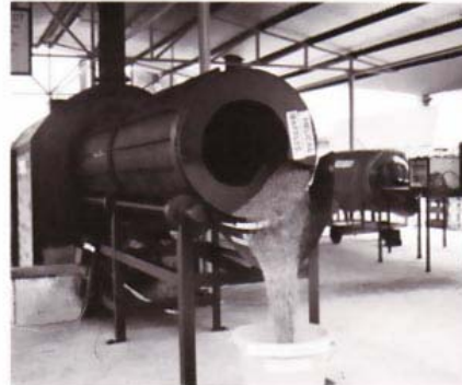
High temperature treatment of paddy in rotary dryers heated by burning rice husk.
