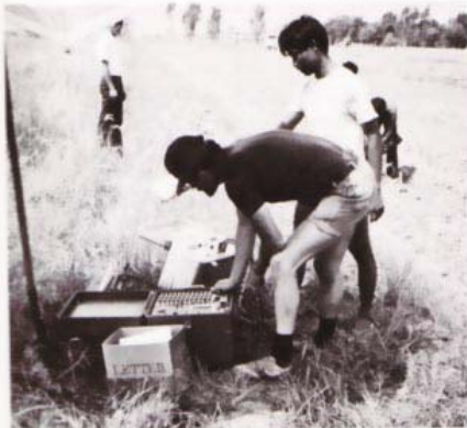
Digital seismograph in high resolution seismic reflection field operations at AIT campus.
