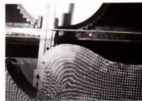
Distortion in soil caused by a single lug.
