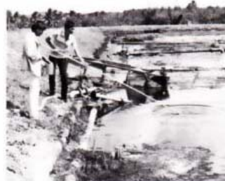
Sampling of effluent storage ponds for analysis at United Palm Oil Mill in Krabi province, Thailand.
