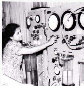
Female enrollment at AIT is growing. Shown above is a female student in geotechnical engineering adjusting a pneumatic triaxial compression apparatus.
