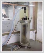
Modified Discharge Capacity Tester
