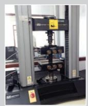
Universal Testing Machine with hydraulic grip and computer system
