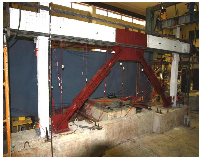
Picture 1a: (above) A scale-down physical model of reinforced concrete frame with buckling restraint braces (BRB). BRB is one of seismic retrofit measures to be considered in this study
