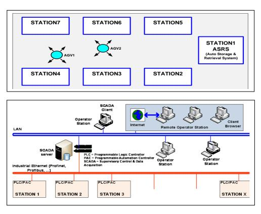
Figure 1. Simplified Horizontal and Vertical Layout of the Laboratory
