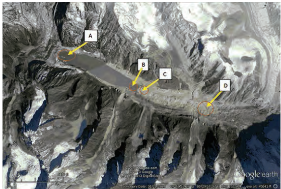
Image of Tsho Ralpa Glacial Lake and Trakarding Glacier showing the points of surface temperature measurement via remote sensing.
